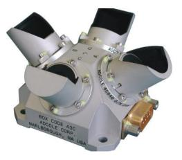
The Coarse Sun Sensor Detector is a single detector model used for applications including solar array pointing, sun acquisition, and fail-safe recovery. The Coarse Sun Sensor Detector is a navigational instrument used by spacecraft to detect the position of the sun.
